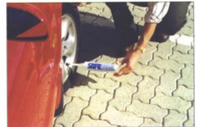
Safeseal is applied by pumping it through the valve of the tyre. It spreads evenly inside the tyre or tube by running the vehicle for 10 km
